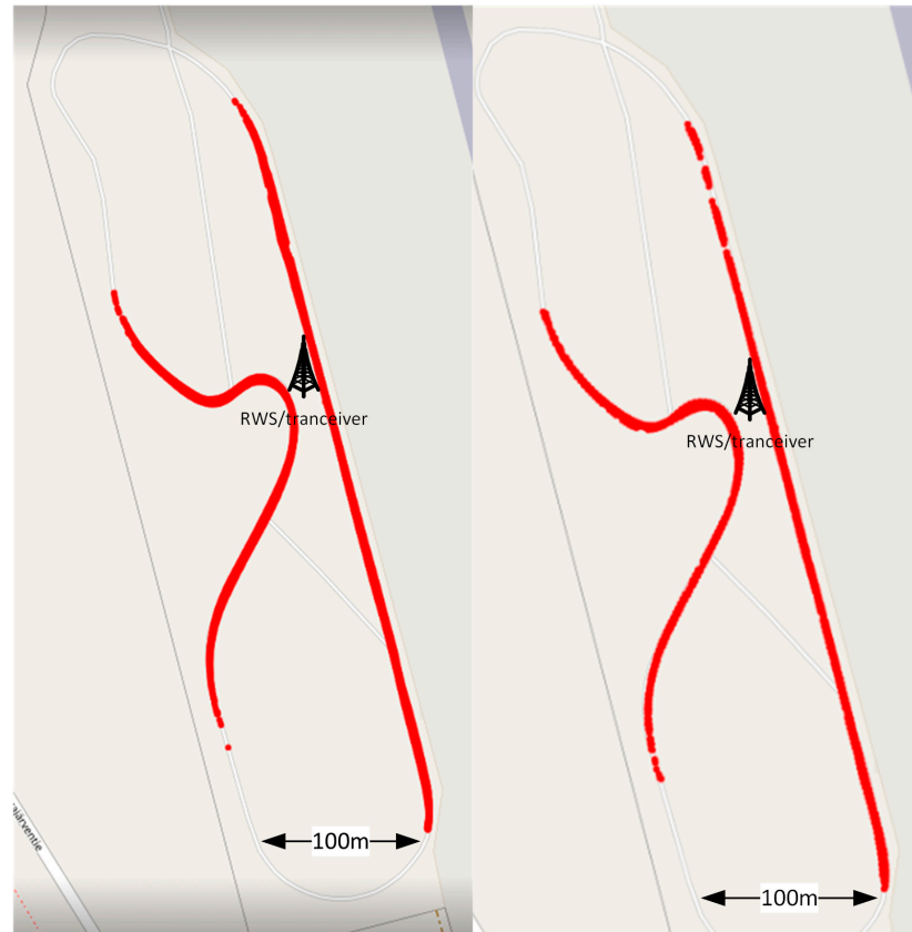
Figure 10. ITS-G5 (left) and C-V2X (right) ranges in test measurements.
